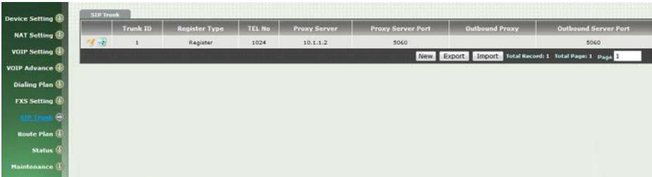
The screenshot shows a web-based configuration interface for SIP Trunk. On the left is a vertical navigation menu with options: Device Setting, NAT Setting, VOIP Setting, VOIP Advance, SIP Trunk (highlighted), Dialing Plan, FXS Setting, Route Plan, Status, and Maintenance. The main content area is titled 'SIP Trunk' and contains a table with the following data:
